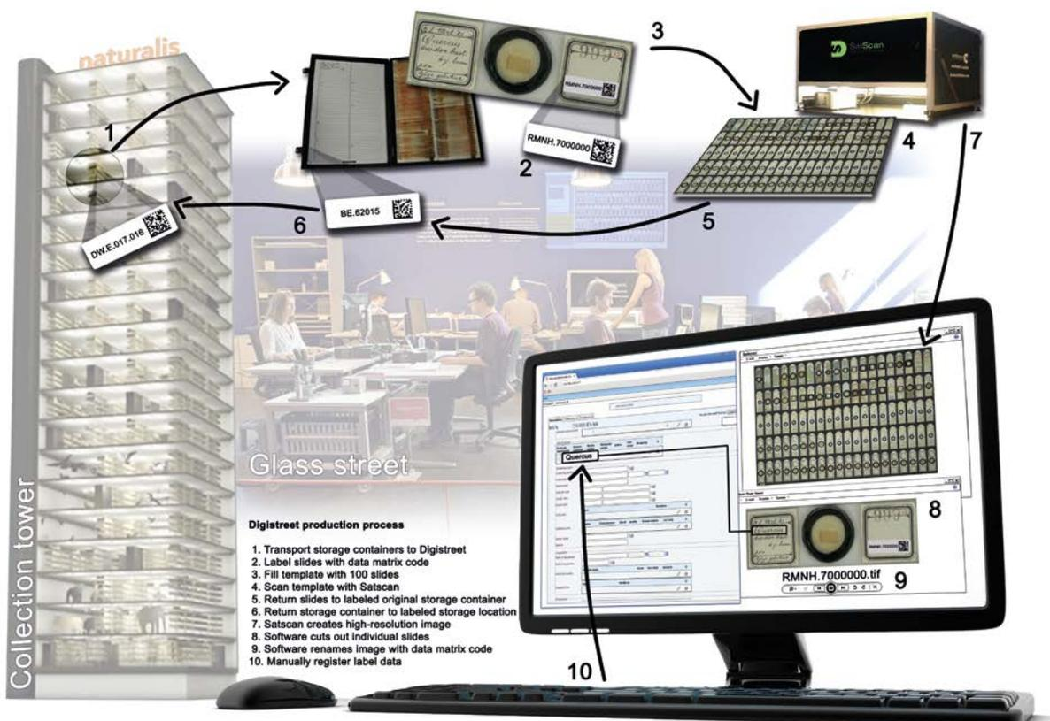
Fig. 2. Schematic representation of the Glass Street production process. Illustration: Ben van Arkel.
